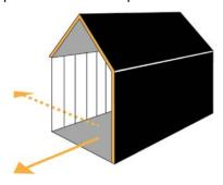
The structure consists of four girders with a rafter. The frame of the fully glazed west façade is detailed out of sight by placing it in the zone of the rafters.
